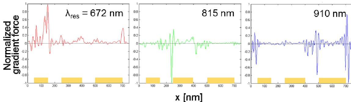
Figure 2. Normalized gradient force calculated from the localized light field for the nanodisk array at the resonant wavelength. It is clear shown that a smaller disk is associated with the highest gradient force at a shorter wavelength.
