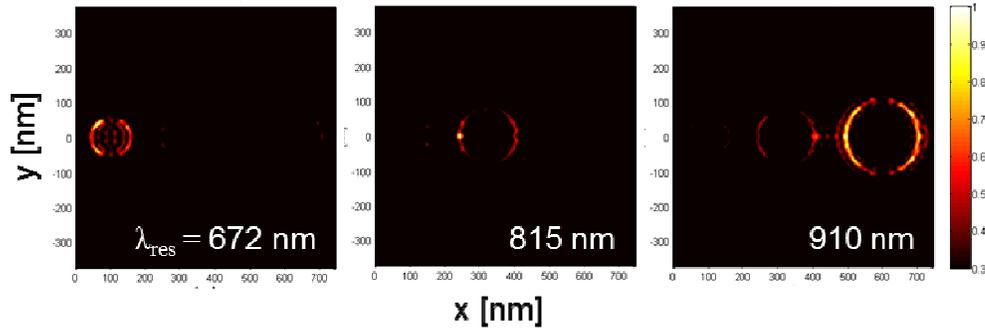
Figure 1. Near-field distribution of the nanodisk array at the resonant wavelength. Color bar represents normalized light intensity. Incident light is  $p$ -polarized (along the  $x$ -axis).
